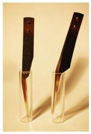
Trimmed forceps (on left) easily reaching bottom of tube. Untrimmed (on right) denied full access, leading to frustration and despair.
