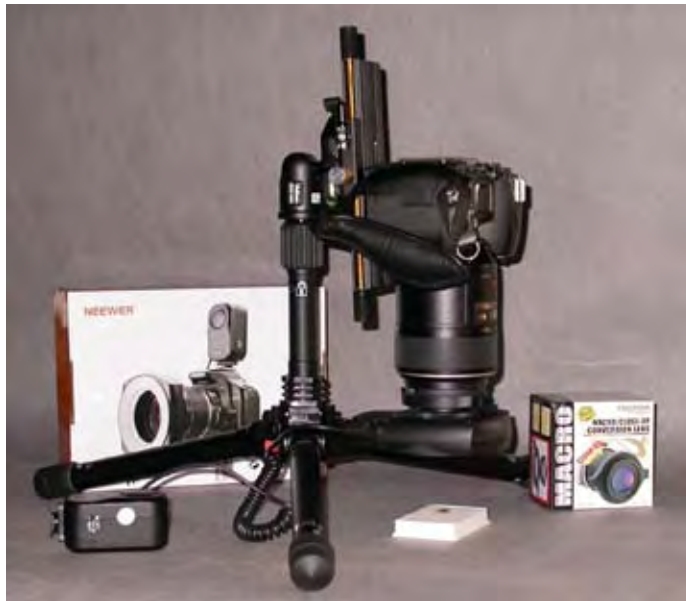
A basic macro stand: tripod by Velbon, focussing plate by Manfrotto, ring lighting by Neewer, clip-on 4.8 diopter close-up lens by Raynox, background by Wickes.
